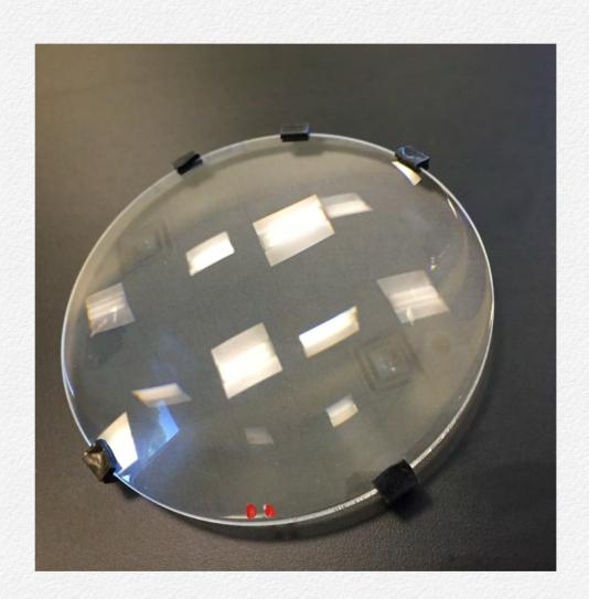
Any lighting instrument using a lens in the theatre is termed a **SPOT LIGHT**, however, not all lighting instruments that create a concentrated beam of light are spotlights. A lens being the requirement for this designation...
