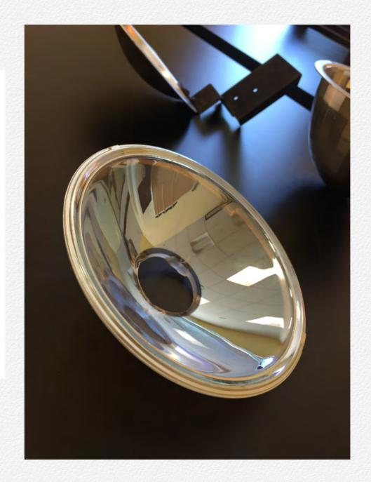
Ellipsoidals (elliptical) The Ellipsoidal reflector was invented to increase efficiency. has 2 foci. Newer reflectors use flatted segments to get a smoother field.
