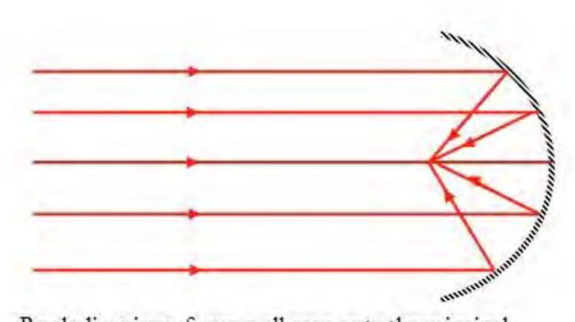
Parabolic mirror focuses all rays onto the principal focus, without spherical aberration.
