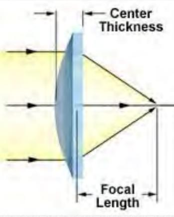
A STEP LENS takes this functionality and by stepping the plano side away, allows the lens to have less mass (less glass and less weight) and greater bending power.
