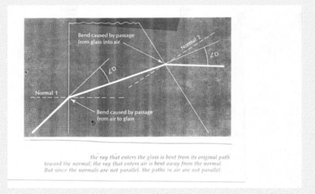
As the angle between the normal at entry and the normal at exit differ, an opportunity arises to control or focus light by creating lenses. Lenses can bend light to concentrate it at an area that is a concentrated point or a focal point.
