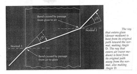
def: NORMAL - a normal is an imaginary line perpendicular to the surface at the point of incidence.
