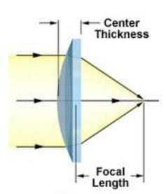
The principle type of lens is called a "PLANO-CONVEX" lens which describes the two sides of the lens
