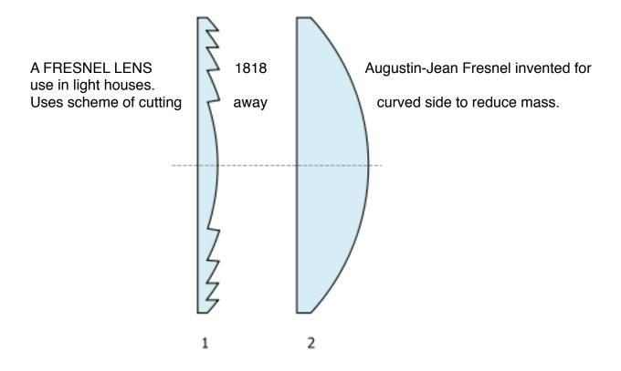
Comparison of a Fresnel lens (left) and a "conventional" plano-convex lens (right). As can be seen, the Fresnel lens simulates the shape of the conventional lens using individual "facets" (also referred to "ridges" or "grooves") - each of which contain a portion of the lens's overall figure. The grooves of the lenses described on this page face "outwards", away from the focal plane.
