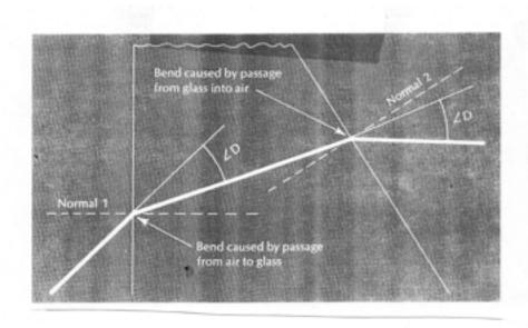
the ray that enters the glass is bent from its original path toward the normal; the ray that enters air is bent away from the normal. But since the normals are not parallel, the paths in air are not parallel.
